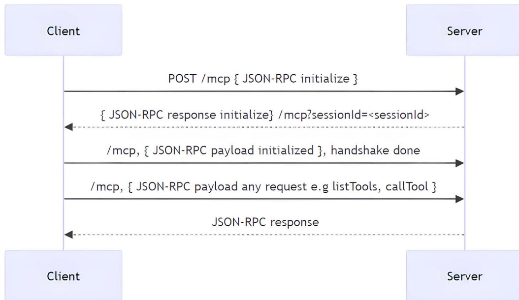
Figure 2.6 – Streamable HTTP flow
