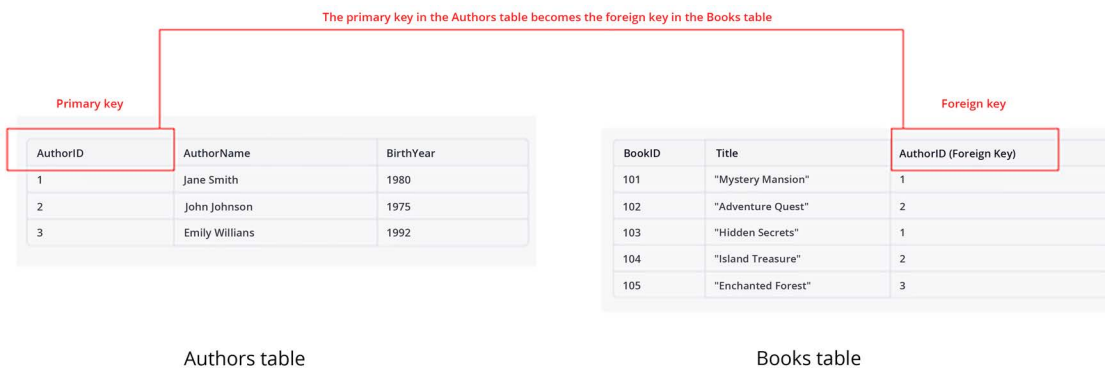
Figure 8.1: An example of the relationship between two tables in a database
